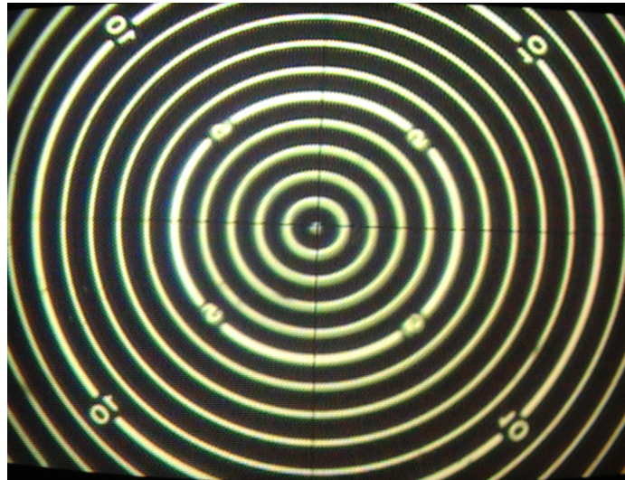
Figure 4.10. The Davidson Optronics D-275 autocollimator object and eyepiece reticle pattern as seen by the CCD camera through the eyepiece and displayed on a CRT monitor. The object reticle obscuration creates the transmitted concentric ring pattern and the eyepiece reticle obscuration makes the cross hairs pattern. Each concentric ring measures the angle of a flat, reflective surface at intervals of one arc minute (two arc minute input field angle). With the crosshairs centered on the dot, the light into the scope is parallel to the optical axis within two arc seconds [16].
